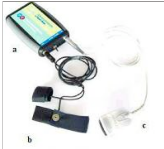
Figure 2. (above) GSR/HR Sensor Module: a) the control box; b) the Skin Conductance Response sensors; c) the Blood Volume Pulse sensor.
